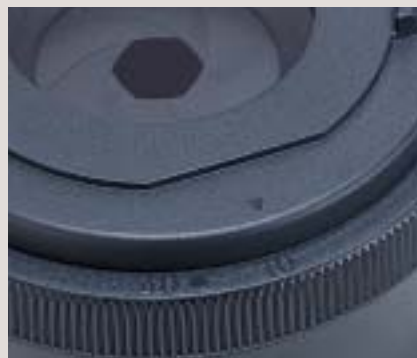
Field diaphragm with position-guide markings
